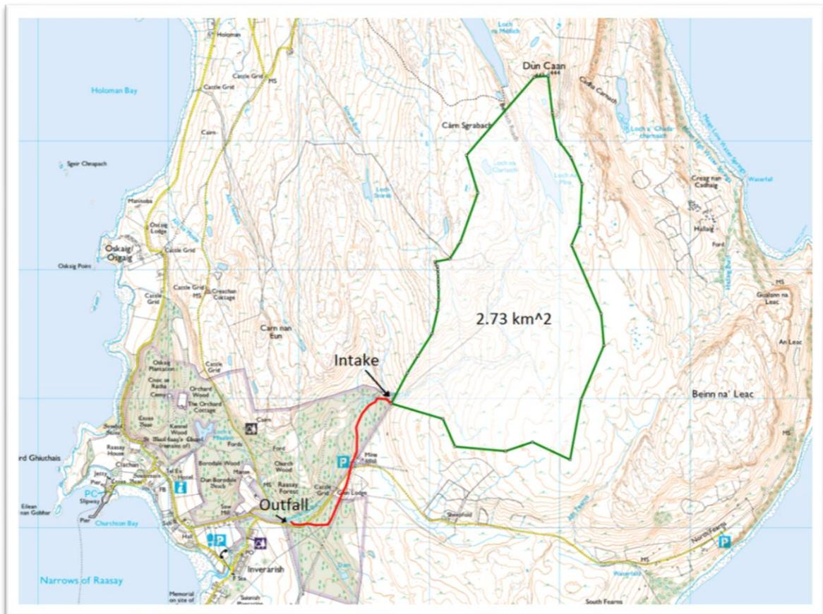
Figure 1: Map of catchment area and suggested penstock route for single intake arrangement.
