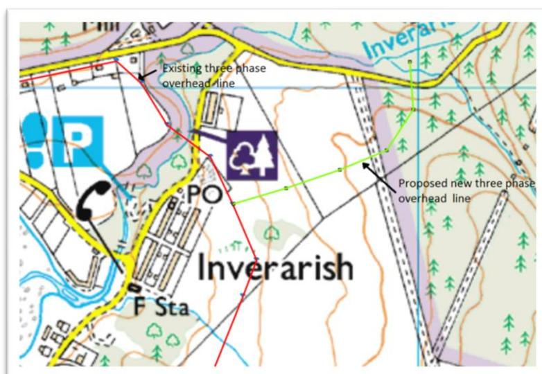
**Figure 9: Map of existing three phase overhead electricity line with proposed spur for hydro scheme connection.**
